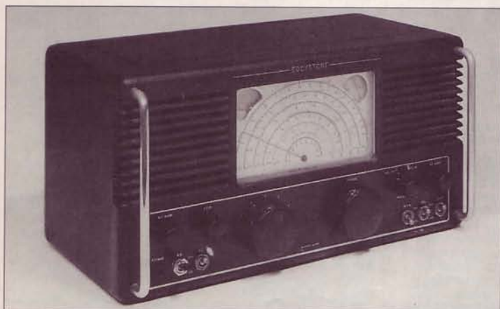
Fig. 1: The Eddystone Model S680, a 15-valved five band 480kHz to 30MHz receiver introduced in 1949 was housed in an aluminium die-cast case.
