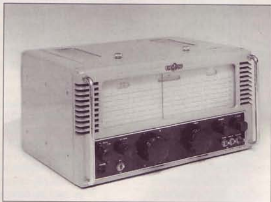
Fig. 4: The Eddystone 770R v.h.f. receiver. This 19-valved set covered 19 to 165MHz in six bands and was introduced in 1953.
